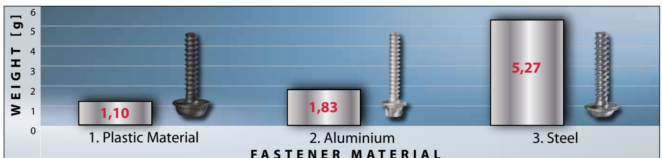
Weight comparison of the screw material
